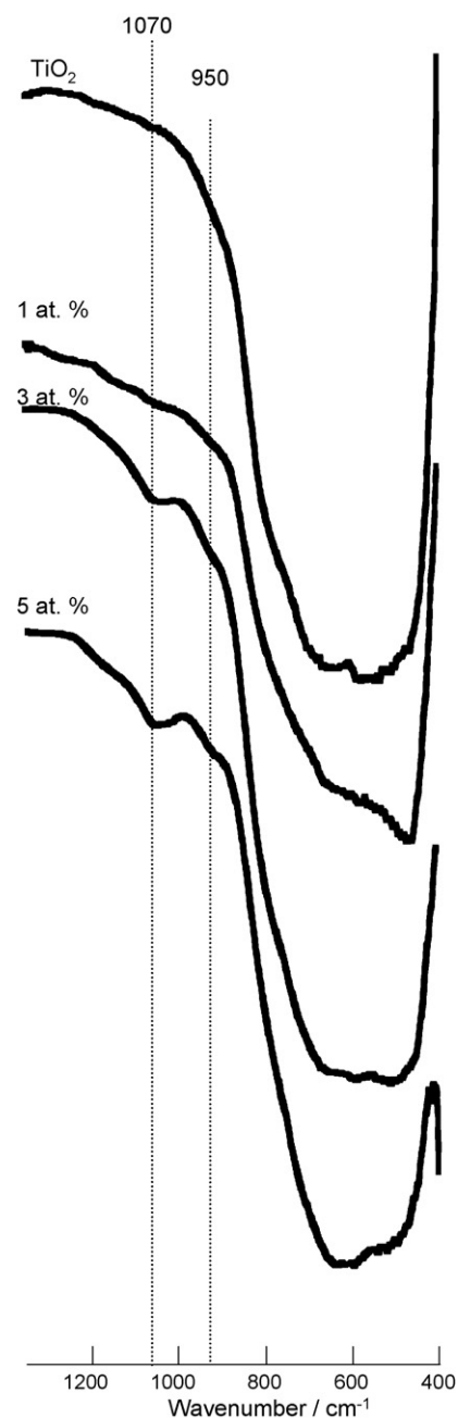
Fig. 2. IR spectra of TiO 2 and silica-modified TiO 2 calcined at 600 °C for 2 h; 1, 3, and 5 at.% Si were added in Si–TiO 2 .
